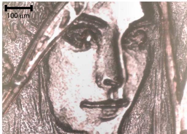
Figure 10. Detail of machined grayscale image 6 . Parameters: \lambda=532\text{nm} , \delta=3\mu\text{m} , PRF=1\text{MHz} , average laser power 1.2W, image size 512 \times 512 points or 1.5 \times 1.5\text{mm} , process time for one layer 1.2s, overall process time 2min
