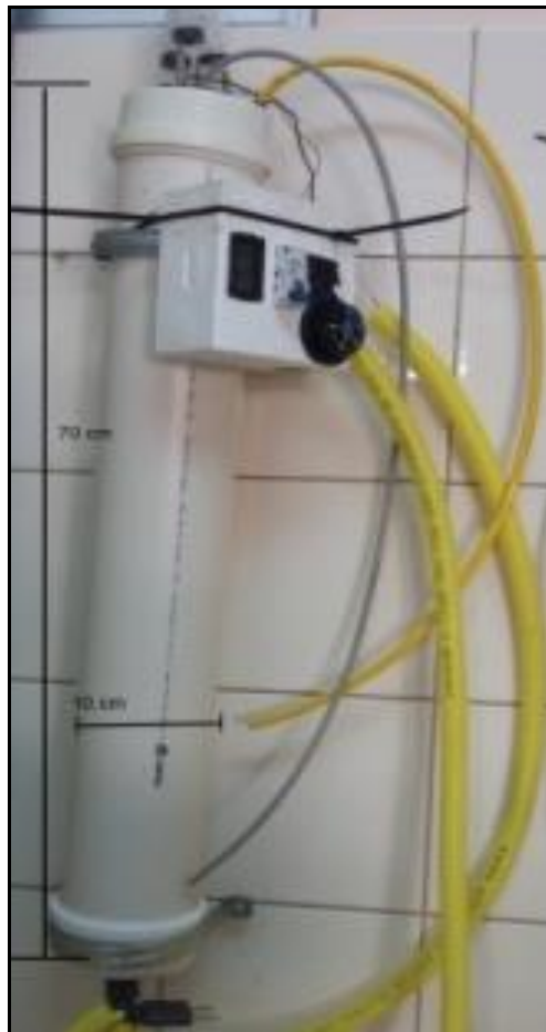
Figure 2 - Alternative airlift bioreactor made of PVC material
