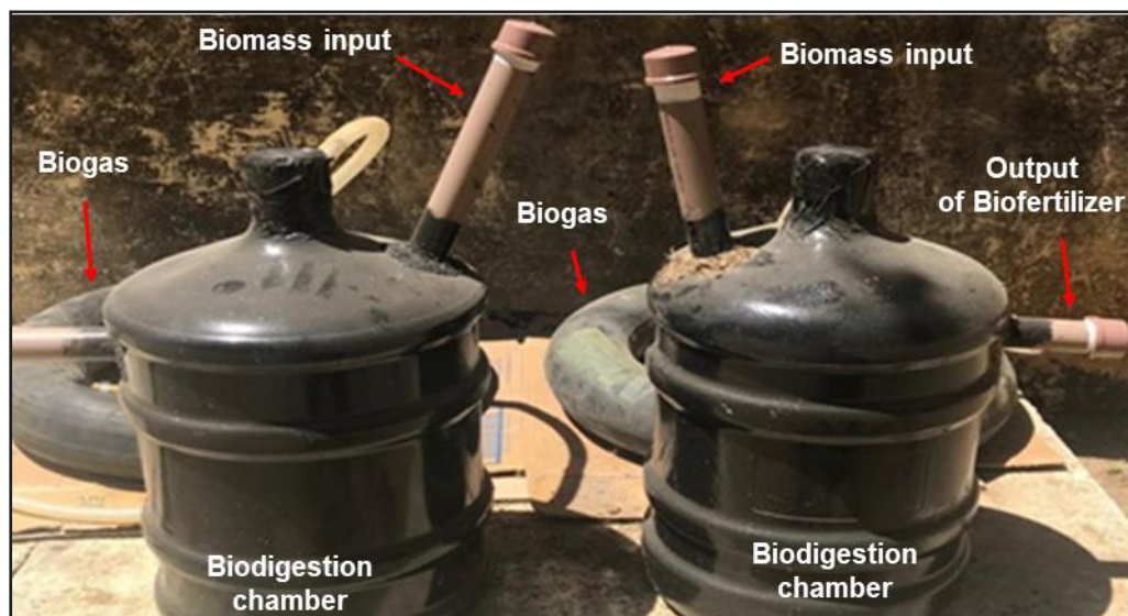
Figure 1– Biodigesters in batch: Homemade biodigesters made of 20 L water bottle, at International Integration of Lusophony Afro - Brazilian University (UNILAB by its name in portuguese), Redenção, Baturité Massif, Ceará
