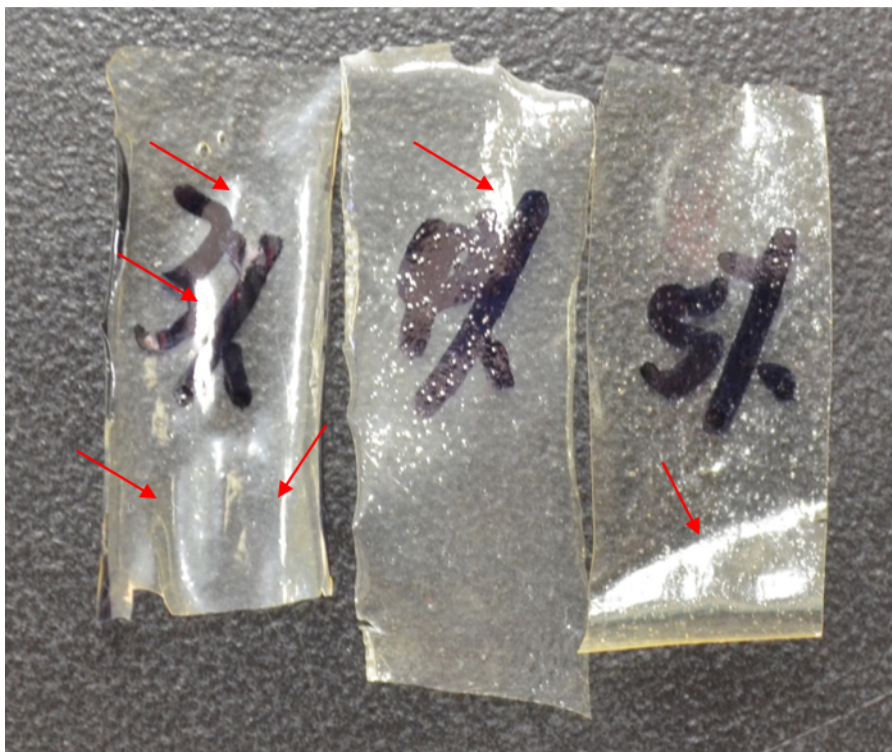
Figure 2-9: Picture for chitosan films after they were crosslinked and dried. The red arrows point to the wrinkles on the film.
