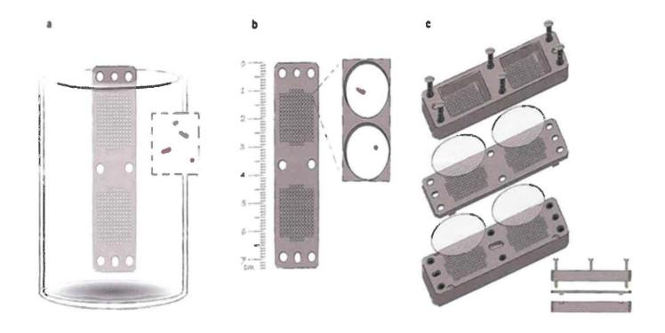
(a & b) sample illustration of how the iChip is placed in suspension to capture single cells per each through-hole; (c) two outer plates are fastened to the center plate in the assembly of the iChip. Adapted from: Ling LL, Schneider T, Peoples AJ, Spoering AL, Engels I, Conlon BP, et al. A new antibiotic kills pathogens without detectable resistance. *Nature*. 2015 Jan 22;517(7535):455-9. Used with permission of the authors.
