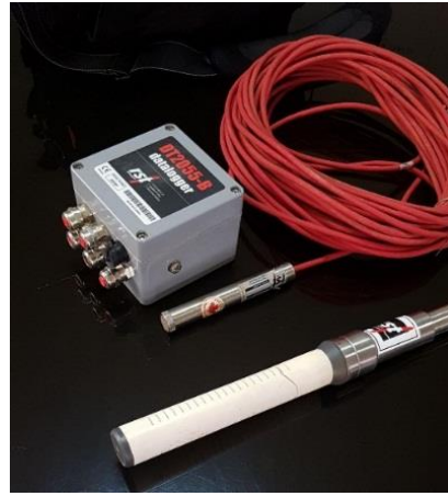
Figure 3. Piezometric Instrument and Data Logger Set
