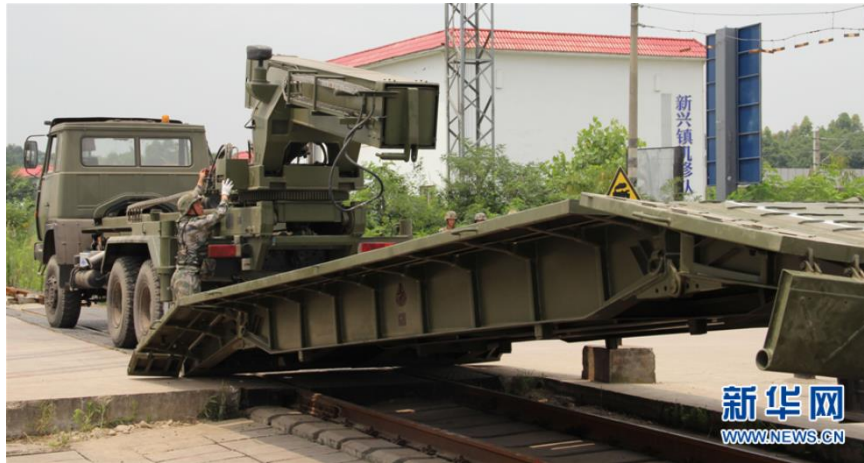
Image 10: A vehicle-mounted railway field platform used during the “Firepower-2015” trans-regional exercise. 122
