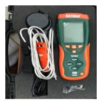
Fig. 4. Light metre used for measuring daylighting (0 lux–400 Klux).
