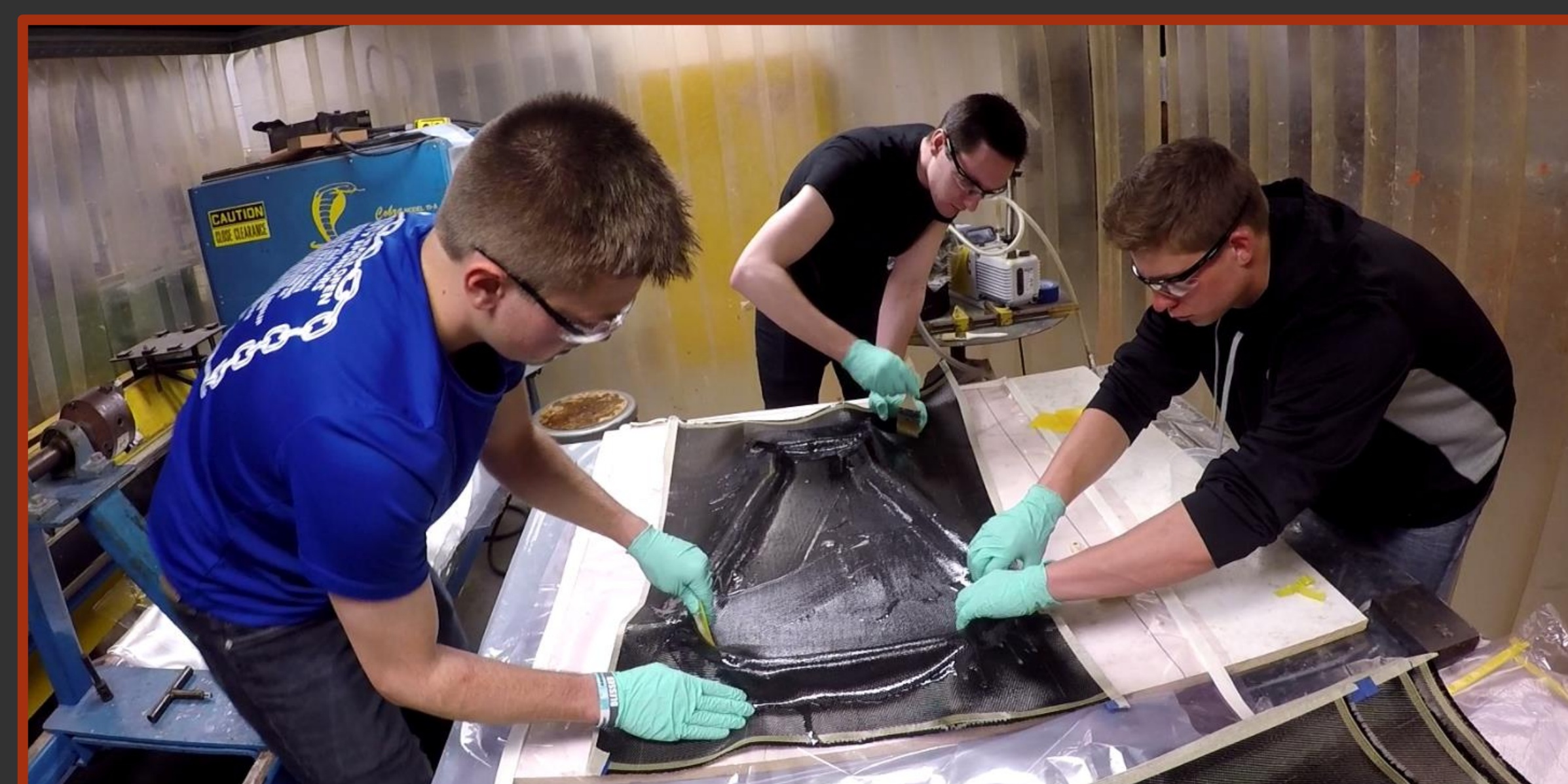
Figure 8: Draping Method Used in Making the Base
