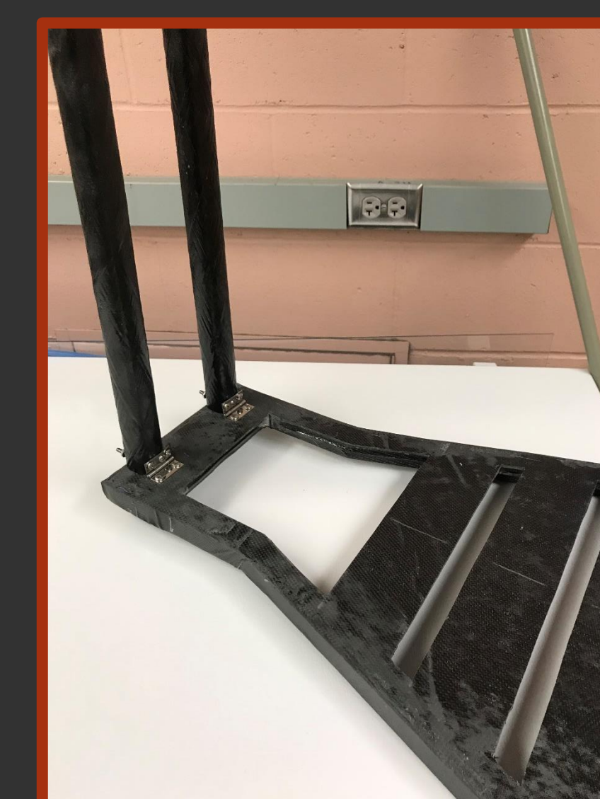
Figure 7: Assembly of Base and Vertical Bars
