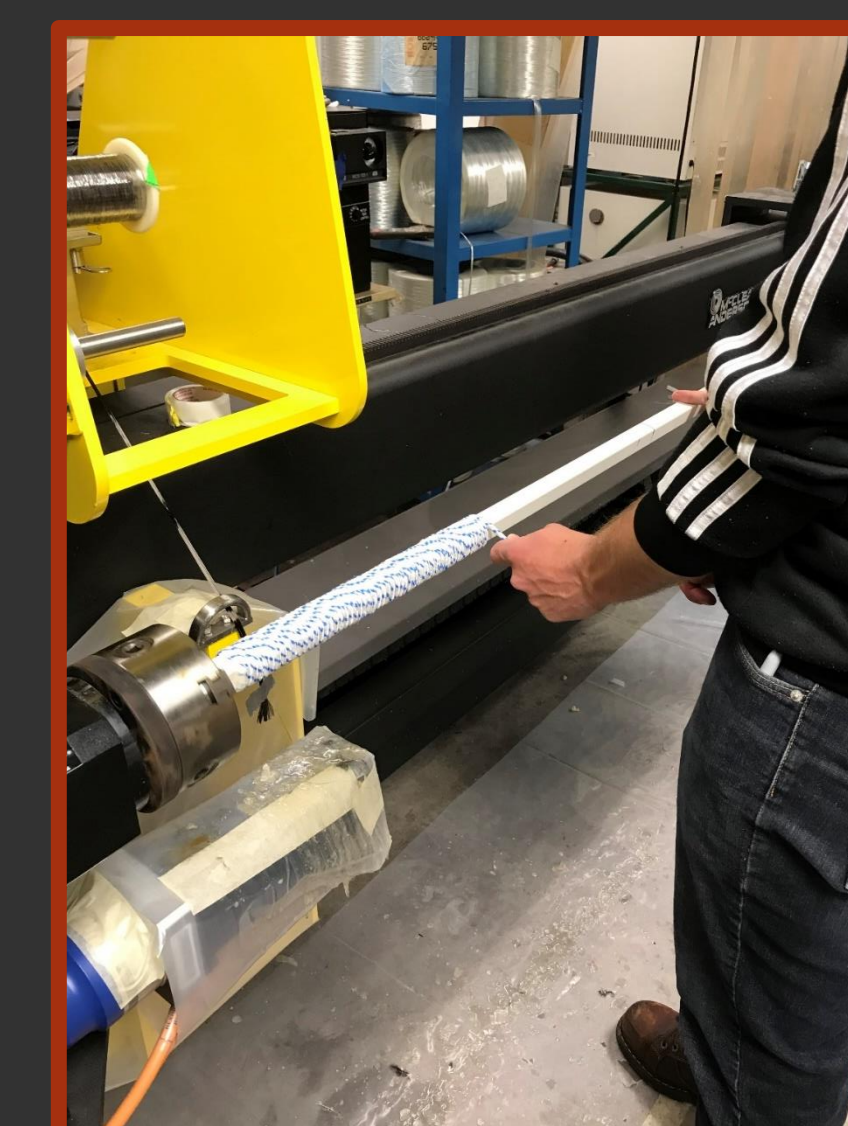
Figure 4: Filament Winding of Vertical Bar
