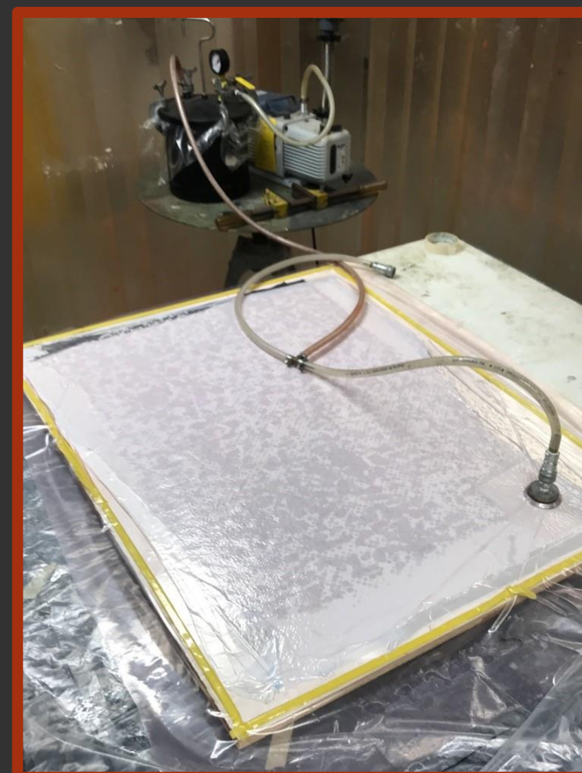
Figure 1: Vacuum Bagged Base Plate
