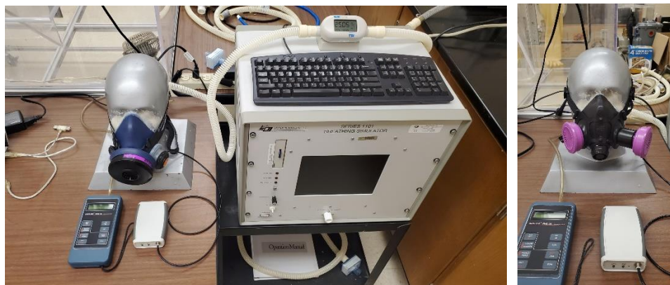
Figure 3.9: Sundström (left) and North (right) constant flow evaluation setup
