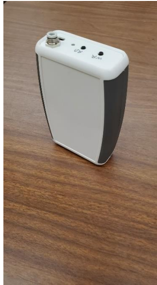
Figure 3.1: S.E.A. Pressure Data Logger Unit
