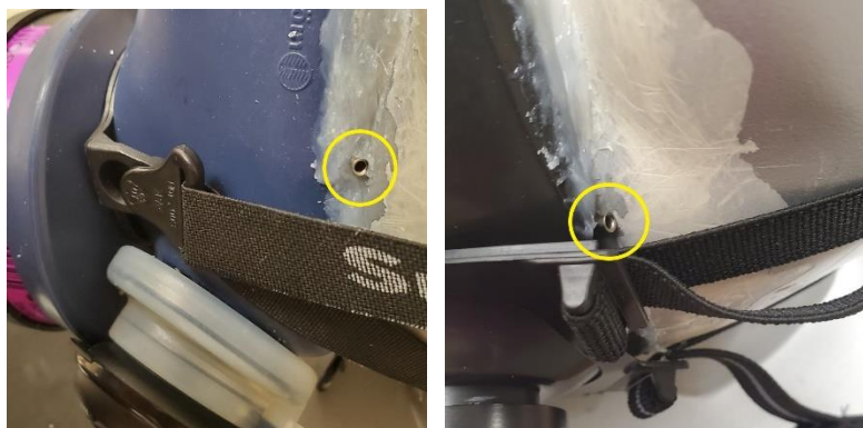
Figure 3.10: Leaks introduced to Sundström (left) and North (right) respirators
