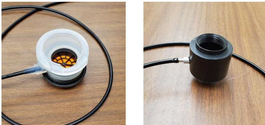
Figure 3.3: PDL connection adapters for Sundström (pictured left) and North (pictured right) respirators.
