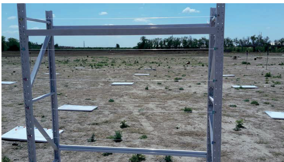
Fig. 3. Frame holding the line collectors for airborne drift, metal plates supporting the petri dishes in the background
