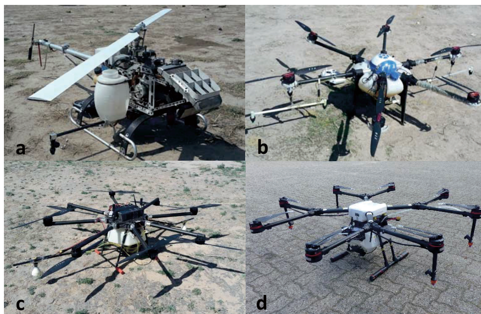
Fig. 1. UAASs involved in the study (a – 1 rotor, b – 6 rotor, c – 8 rotor (TTA) and d – 8 rotor (DJI))
