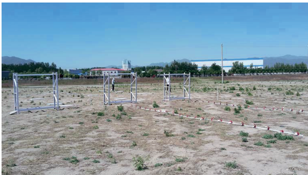
Fig. 2. Test site with experimental arrangement for spray drift measurement. Bars holding deposit plastic cards in front.
