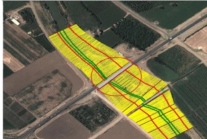
Fig. 4. Cross sections to determine the depth of scouring of bridge piers.
