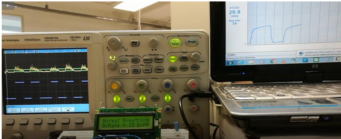
Fig. 18. Comparison between respiratory rates measured with the developed device and with capnography device at normal shallow breathing (15 BrPM).
