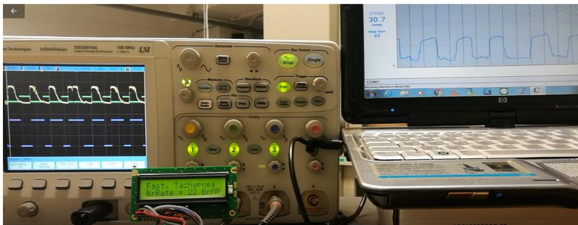
Fig. 19. Comparison between respiratory rates measured with the developed device and with capnography device at fast breathing (22 BrPM).
