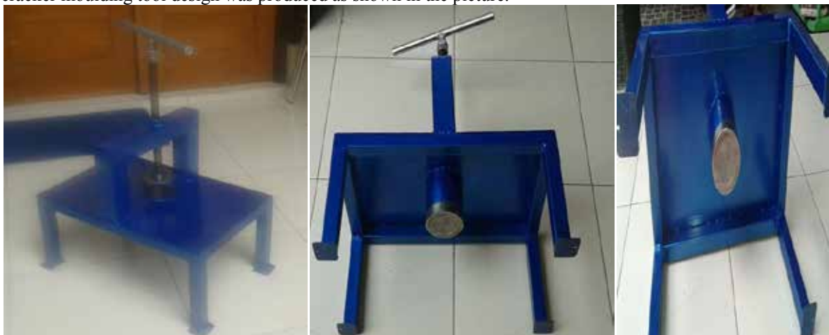
Figure 5. Results of the Design of Noodle Crackers Moulding Tool
