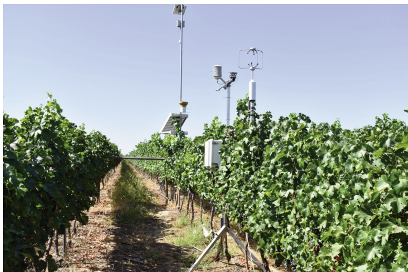
FIGURE 1. A vineyard monitored with an EC system. There is a sonic anemometer at the front, and tools for ET_{ref} measurements (pyranometer, relative humidity, windspeed, temperature, rain gauge), for other atmospheric recordings (solar panels, data logger for soil moisture sensor, heat plate) and data transmission box in the background.
