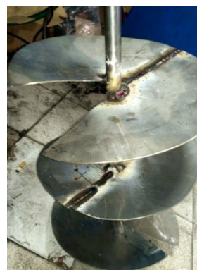
Gambar 4.6 Mixer blades after going through the welding process
