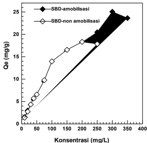
Figure 3 : The influence of solution concentration on Zn(II) biosorption by immobilized and non-immobilized biosorbent (pH Zn solution = 5, volume = 20 mL, mass = 0.1 g, contact time SBD – immobilized = 90 minutes and SB-non immobilized = 45 minutes)
