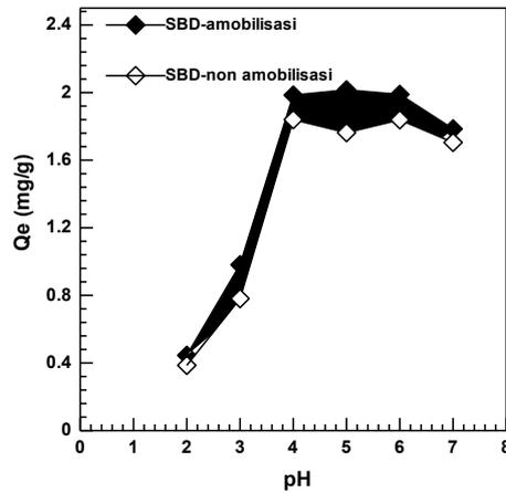
Figure 1 : The influence of pH on solution towards Zn(II) absorption capacity. (Initial concentration =  $10 \text{ mgL}^{-1}$ , volume = 20 mL, mass = 0.1 g, contact time = 60 minutes)
