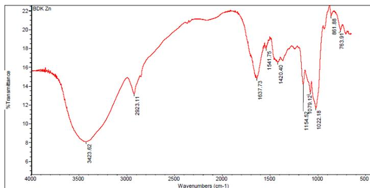
Figure 5 : FTIR Spectra for Ca-alginate immobilized durian seed biosorbent before absorption
