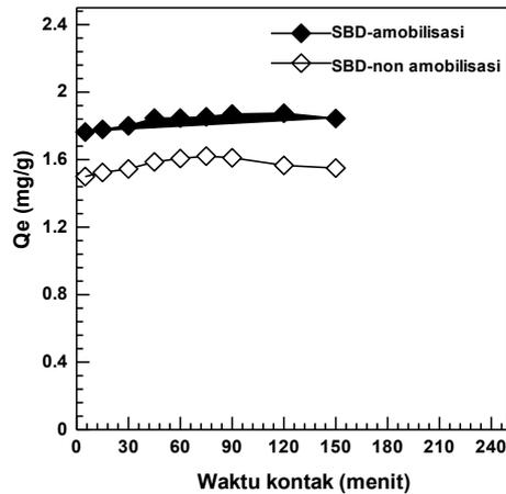
Figure 2. The influence of contact time on Cd absorption capacity, pH 4 at non-immobilized and pH = 5 at SBD-immobilized, biosorbent mass = 0.1 g, initial concentration = 10 mgL<sup>-1</sup>, stirring rate = 150 rpm.
