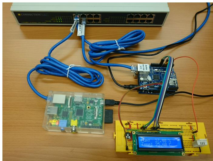
Figure 4. Prototype implementation using Arduino and Raspberry Pi boards.
