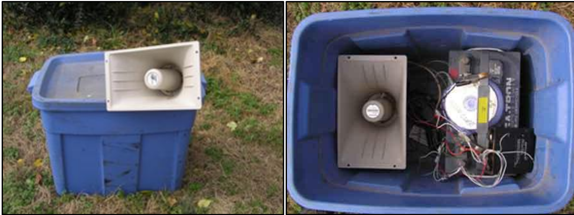
Photos of audio lure components. Photo on left shows components inside plastic container including battery, CD player, amplifier, and bell speaker and connectors. Photo on right shows audio lure in operation with external bell speaker. Photos by Fletcher Smith.
