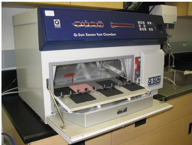
Fig. 2. Q-Sun Xenon Test Chamber for accelerated UV weathering of microplastics.
