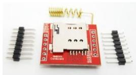
**Gambar 3. Modul SIM 800L Error! Reference source not found.**
