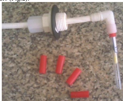
Fig.2: Sampling holders designed for dynamic chamber sampling
