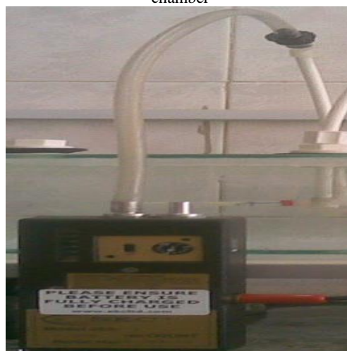
Fig.4: Air sampling train and adsorbent tubes arrangement followed by sampling holders
