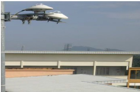
Fig. 4. CMP11 thermopile pyranometers with ISO 9060 Secondary Standard
