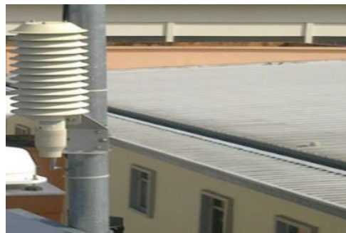
Fig. 6. Temperature & humidity sensor used to measure ambient temperature
