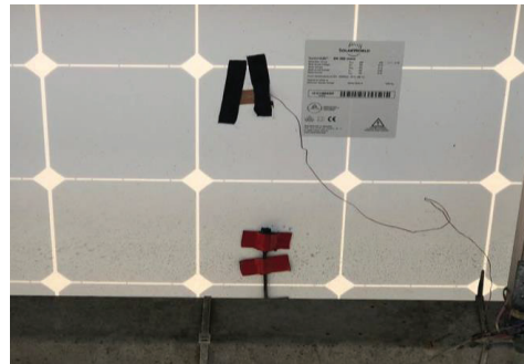
Fig. 5. Thermocouple Sensor connected to monocrystalline PV module at FKE, UTeM
