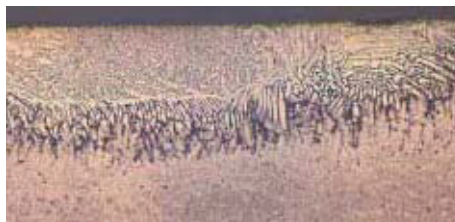
Figure 1 Optical micrograph of the NiTi-NiTi plasma weld [25]
