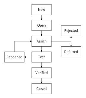
Figure 1: Defect Life Cycle.
