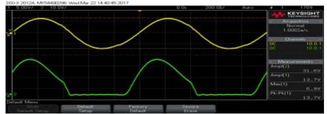
Figure 10: Experimental results of Class E inverter with impedance matching network
