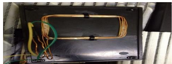
Figure 11: Designed Transmitter Coil
