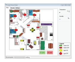
Figure 10: VB GUI Main Tab. To control appliances, click on the named objects on the map
