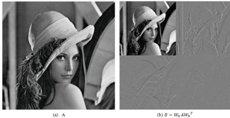
Figure 2. Figure 2(a) Original image and Figure 2(b) Level 1 Haar transform of Lenna image.
