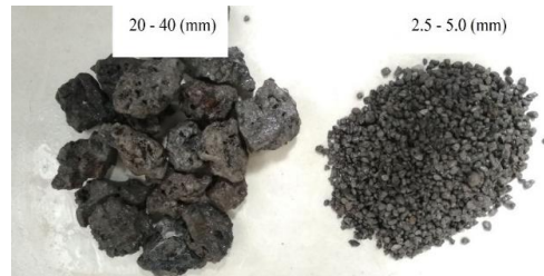
Figure 1. Preparation of two categories of steel slag aggregate: coarse slag 20-40 mm and fine slag 2.5-5 mm.
