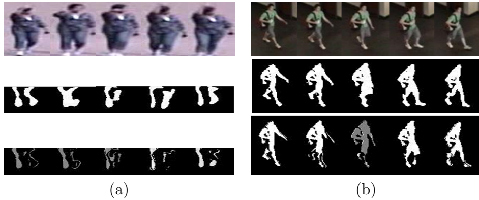
Figure 5.5: GEI features extracted from sample sequences from the 2 datasets, (a) Lower body FDEI from MCID dataset and (b) FDEI from the SAIVT Soft-Bio dataset.
