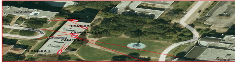
Top View: Cameras mounted around the periphery of PGH to monitor people entering or leaving the building.
