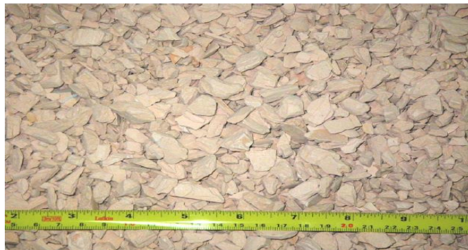
Figure 2: Sinterized Calcined Clay Aggregate (SCCA) after controlled calcination and crushing process.
