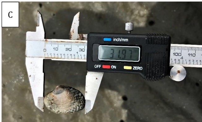
Figure 2-12 Tools for density measurement and size scaling in the present study. After set quadrat with a folding scale, beach sand was dug up and put in a bucket (A), and filtered with 1mm mesh sieve (B). All found clams were scaled their body length with a digital caliper(C).
