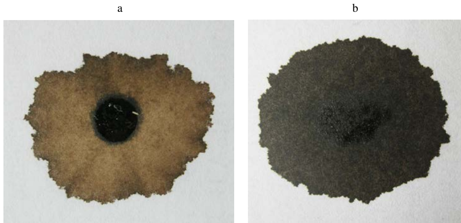
Fig. 4. Photos of the dried drops of the poor quality magnetic fluid and the qualitative one: a – MOT-29; b – MOT-39
