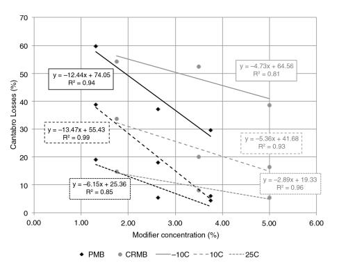
FIGURE 8. Thermal sensitivity vs. modifier concentration.
