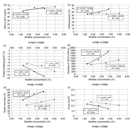
FIGURE 3. Binder properties vs. Modifier concentration: a) Needle penetration; b) Softening point; c) Fraass breaking point; d) Viscosity at 140 °C; e) Elastic recovery and f) Force-ductility.
