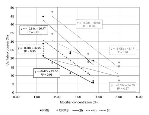
FIGURE 9. Ageing resistance vs. modifier concentration.
