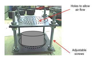
FIGURE 2. Device for ageing process.
