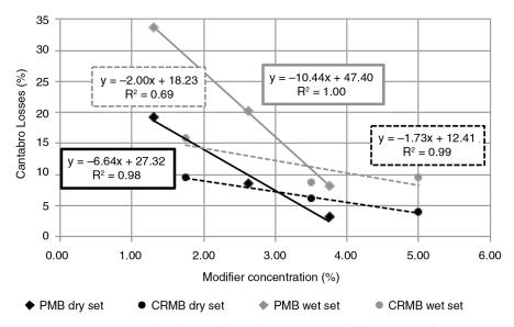
FIGURE 7. Cantabro losses of dry and wet sets vs. modifier concentration.
