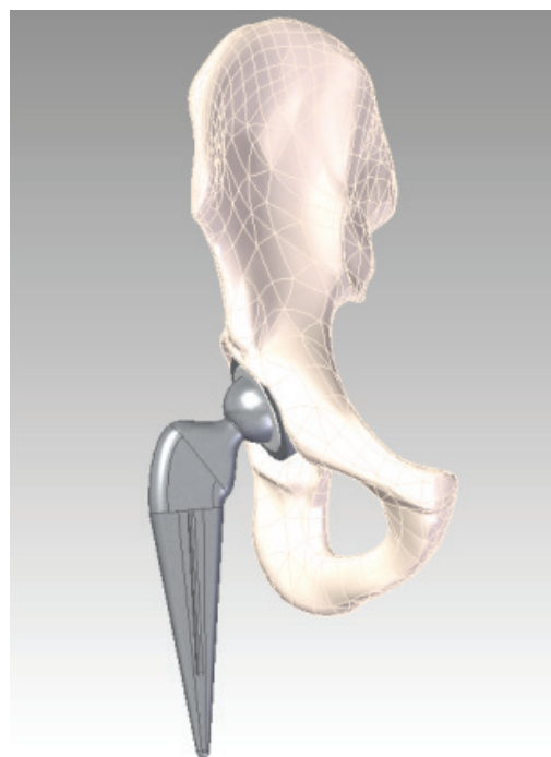
Fig. 6. The pelvic bone with mounted endoprosthesis of the hip joint (front view) [source: own study]
