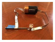
Assist as needed. One idea for conductivity testing is shown here. Aluminum foil folded into strips works well. These can be taped to the battery and the bulb holder for more stability.
