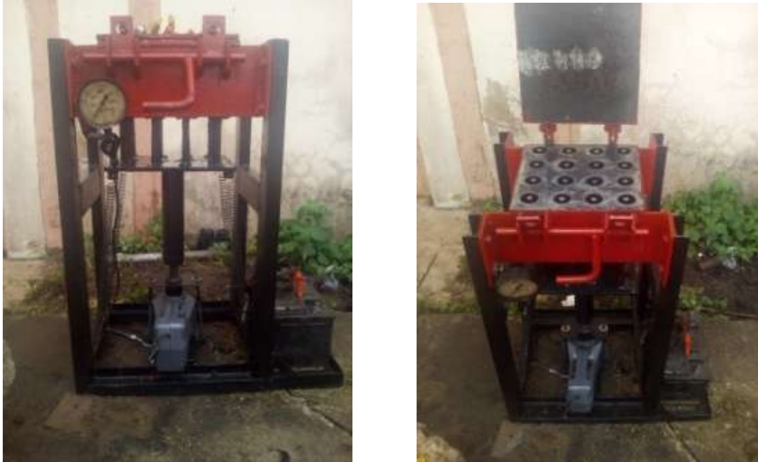
Plate 1: Plan and front view of the hydraulically operated agricultural waste briquetting machine
