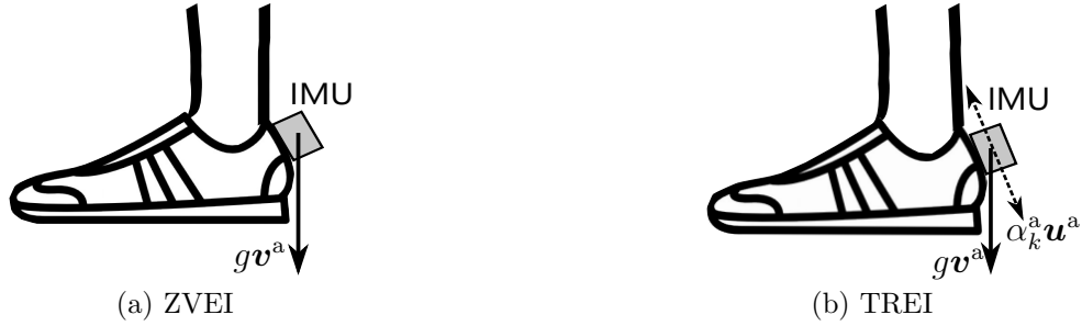
Figure 3.2: Gait patterns. (a) Zero-velocity event intervals (ZVEI) are associated with no movement gait pattern in FOG. (b) Trembling event intervals (TREI) are associated with alternating trembling in the lower extremities gait pattern in FOG.
