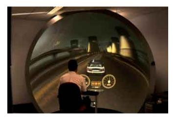
Fig. 9. iDome and car racing game example. While the warped image sent to the data projector (figure 5) appears distorted, the imagery is perfectly correct on the dome surface.
