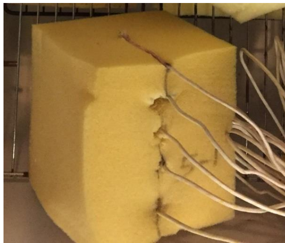
Figure 4-28: Location of Surface Mounted Thermocouples
