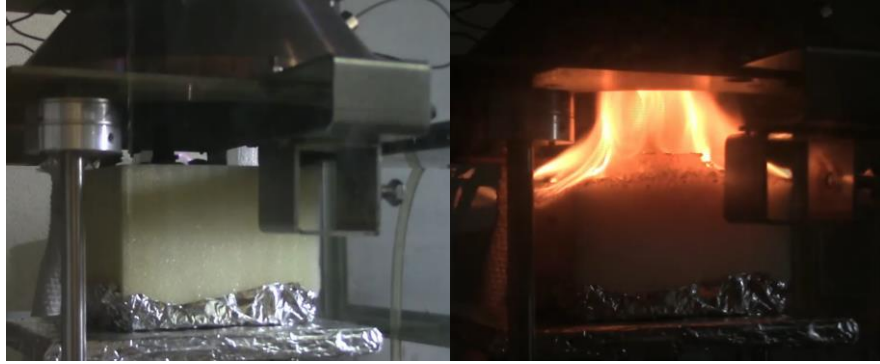
Figure 2-4: Cone Calorimeter Heat Release Rate Density Test
