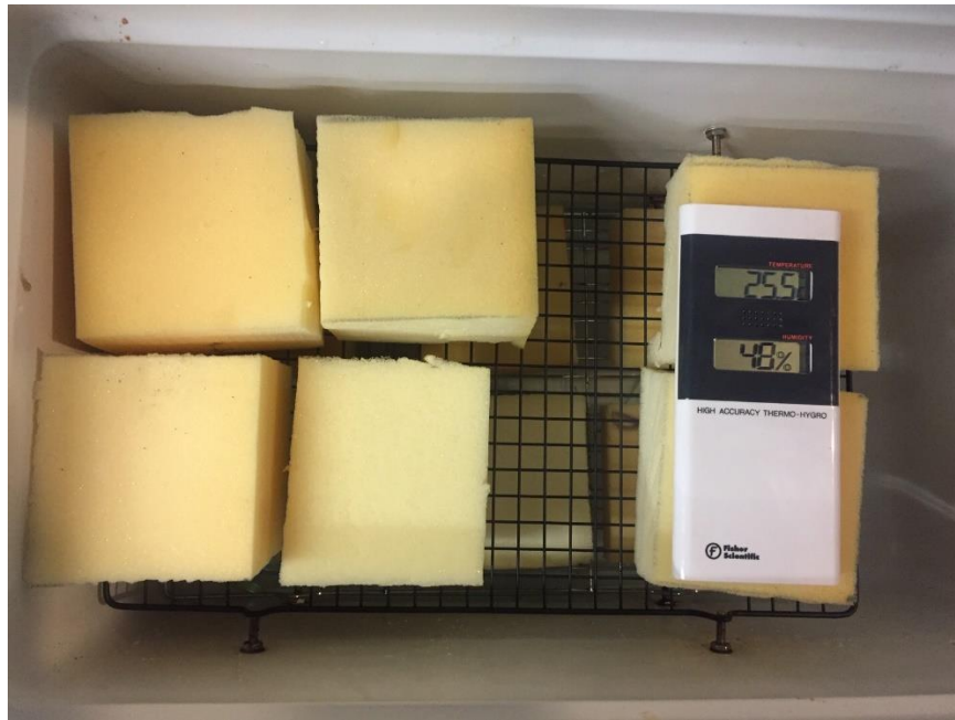
Figure 2-3: Foam Test Specimen Conditioning Cooler
