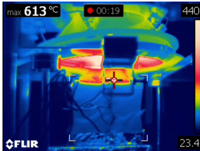
Figure 4-23: Infrared Temperature Measurements for 10 cm Thick Polyurethane Foam Exposed to 10 kW/m 2 Heat Flux (12 s exposure time)
