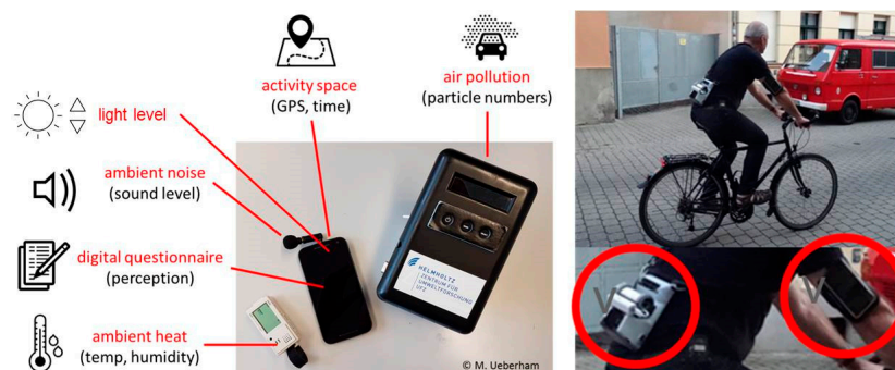
Figure 1. Sensor equipment (left) and study participant wearing the sensors (right).
