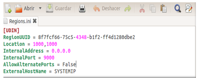
Fig. 2. View of Regions with location, internal address, port and the name UDIN server, Regions ID it is compose for a hexadecimal number unique in the world.
