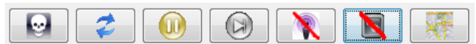
Fig. 5. The NPC control interface. From left to right, Kill agent, Reload logic, Play/Pause agent, Show/Hide agent state,
