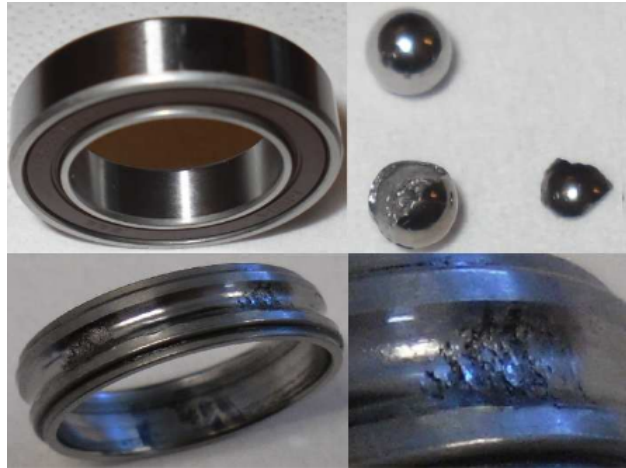
Figure 15: Normal versus degraded bearing components [32]
