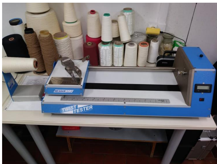
Sl. 20. Torziometar, Twist –T, Mesdan Lab
