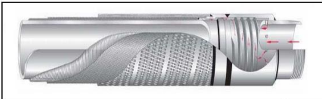
Figure 2-8. ICD helical-channel type (Al-Khelaiwi and Davies, 2007)
