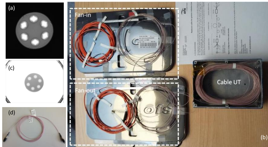
Figure 9: a) Profile of multi-mode, multi-core fiber, b) cable sample connected to fan-outs for radiation testing, c) end-face of multi-core MiniAVIM connector and d) assembled multi-core, MiniAVIM patchcord prototype
