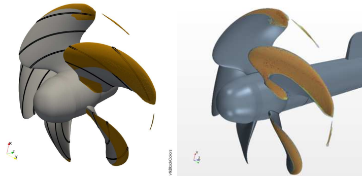
Figure 3.4: Predicted cavitation pattern for propeller A with J = 0.85 , \sigma = 2 by OpenFOAM (left) and Star-CCM+ (right)
