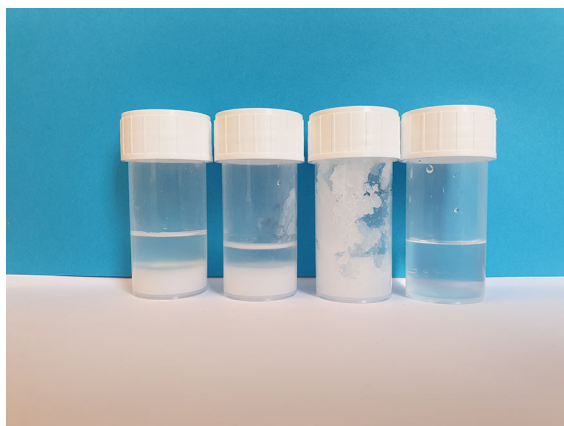
Fig. 1 From left to right: 3 wt% MCC in 2.3 M 50/50 mol.% KOH/TMAH(aq), 2.3 M 50/50 mol% KOH/NaOH(aq), 2.3 M 50/50 mol% NaOH/TBAH(aq) and 2.3 M 50/50 mol% NaOH/TMAH(aq)
