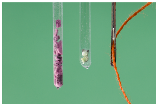
FIG. 9. Photograph of the samples of \text{NaCoF}_3 (left) and \text{NaNiF}_3 (right) post-perovskite samples used for the neutron powder diffraction experiments on the upgraded Polaris. The diameter of the silica glass capillary tubes in which the sample is contained is 1.5 mm. Reproduced with permission from Lindsay-Scott et al. , J. Appl. Crystallogr. 47 , 1939 (2014). Copyright 2014 International Union of Crystallography. Photograph: STFC.
